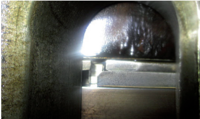
Fig. 1: Top piston ring with a broken gas-tight lock
